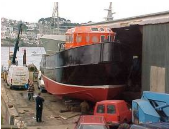
Polmear being Built at Toms Yard Polruan. Framed up
