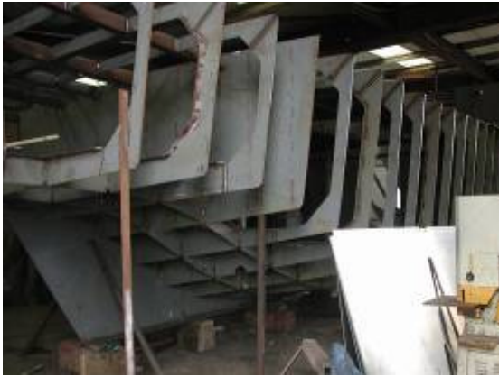
Polmear being Built at Toms Yard Polruan. Framed up
